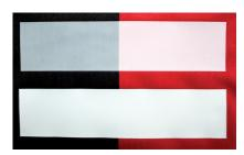
Many users forget that most of the fabrics for sportswear are made of polyester which is coloured with sublimation ink. During the heat transfer not only the hotmelt but the sublimation pigments are activated as well. In time the sublimation pigments seep through the flex and even though the Flex looked perfect directly after the transfer, it now shows a certain discoloring.
